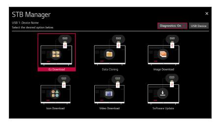
5. If more than one USB memory device is currently connected to the STB, be sure to select the USB device that contains the applicable video file. If necessary, use the arrow keys on the Installer Remote to select/highlight the USB Device button in the top right corner of the screen and press OK. Then, use the Up/Down arrow keys to select the appropriate USB device from the pop-up list of USB devices.
