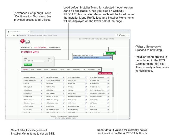
**Note:** The Pro:Centric tab enables you to set up Pro:Centric-specific parameters, the LAN tab enables you to set up a variety of LAN features, and the Wi-Fi Zones tab enables you to set up Wi-Fi Zones. Refer to the *Cloud Configuration Tool User Guide* for further information. Also, see Reference section, "Using the STB's Zoning Features," for additional information on Wi-Fi Zoning.
