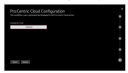
2. Use the arrow keys to select **Search** and press **OK** to verify the installation code. When the installation code is verified, the "Search" button becomes a "Next" button (you also will see a "Server Found" message below the Installation Code field). Select **Next** and press **OK** to continue.
