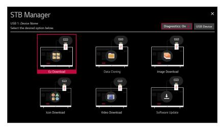
5. If more than one USB memory device is currently connected to the STB, be sure to select the USB device that contains the applicable image file(s). If necessary, use the arrow keys on the Installer Remote to select/highlight the USB Device button in the top right corner of the screen and press OK. Then, use the Up/Down arrow keys to select the appropriate USB device from the pop-up list of USB devices displayed at the top of the screen.
