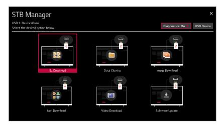
6. If more than one USB memory device is currently connected to the STB, be sure to select the USB device on which you wish to save the Clone file. If necessary, use the arrow keys on the Installer Remote to select/highlight the USB Device button in the top right corner of the screen and press OK. Then, use the Up/Down arrow keys to select the appropriate USB device from the pop-up list of USB devices.
