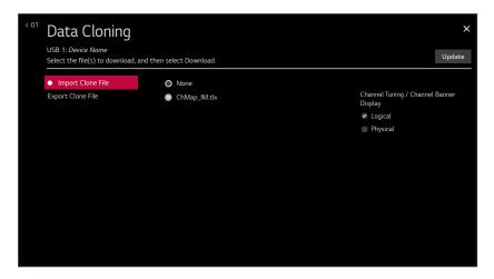
10. Use the arrow keys on the Installer Remote to select/highlight the ".tlx" file to import, and then press **OK**.
