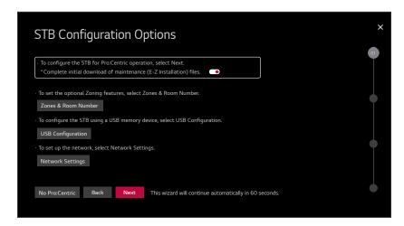
**Note:** If there is no user action in this screen within one minute, the wizard will automatically continue to the next configuration step. If you would like to exit the wizard at any time, use the arrow keys on the Installer Remote to select/highlight the ❸ button at the top right of the screen, and then press **OK**. In the exit confirmation screen, select the appropriate "Exit" option (see also note below), and then press **OK** once more on the Installer Remote.
