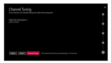
• If you would like to initiate an automated channel scan (i.e., a search for all available digital and analog channels), use the arrow keys on the Installer Remote to select the RF tuning band field, and select the appropriate option. Then, press **OK**. Next, select the **Channel Tuning** button at the bottom of the screen, and press **OK**.
